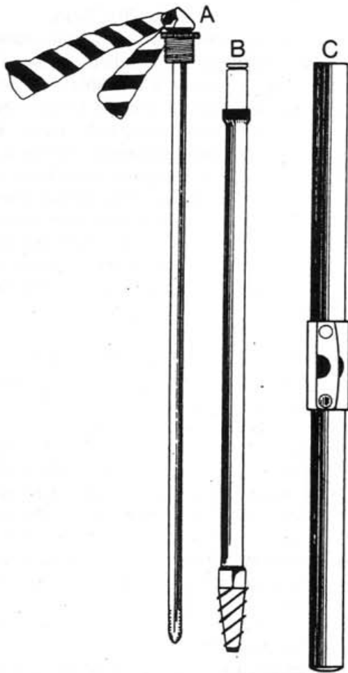
Figure 1. An increment borer has three pieces: the extractor (A), the borer bit (B), and the handle (C). Flagging the extractor makes it highly visible to help avoid losing it or stepping on it.
