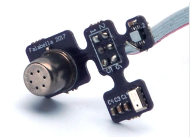
Fig. 4. Peripheral sensor bundle with gas, relative humidity, and barometric altitude sensors mounted.
