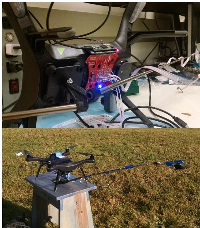
Fig. 5. Top: sensor development board connected to the ventral side of the UAS, alongside the fiberglass booms and ribbon cable. Bottom: Fully-equipped UAS displayed before conducting a sample flight
